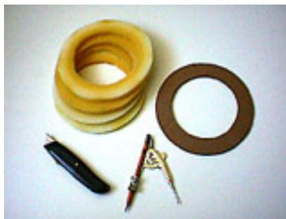
A cutting guide ring is first cut out of cardboard. The outside of the guide ring should be approximately the same as the inside diameter of the mute. The inside diameter of the guide ring should be about 1-1/4" less than the outside diameter.
