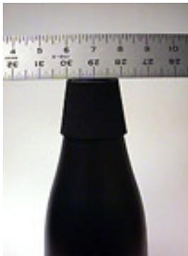
The width of the top of the rubber is 1.99" and only the leading edge contacts the bell of the trombones used in this test. As demonstrated in the section on weight and balance, the large throat diameter causes the center of gravity of this mute to extend well beyond the bell with a typical small or medium bore horn. It will fit better in a bass trombone, or a large tenor bell.
